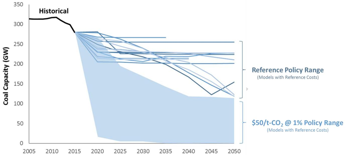
**Figure 16. Coal capacity (GW) by model and time under alternate policy scenarios.** Values shown for the reference technological scenario only.
