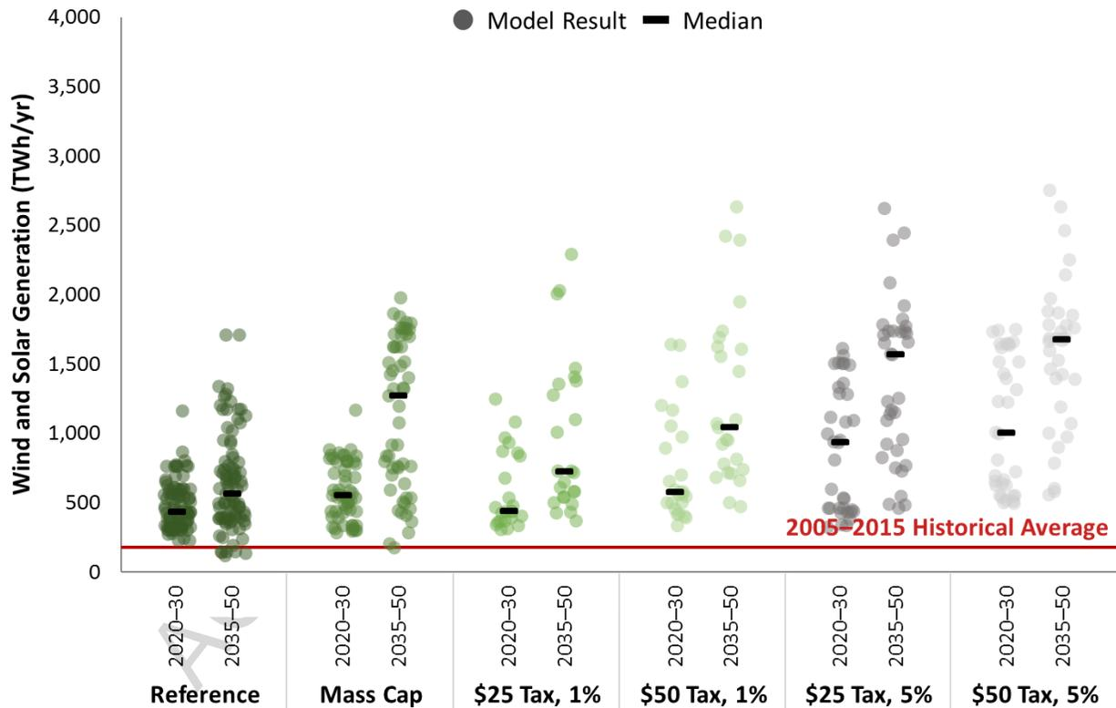
**Figure 3. Annual wind and solar generation (TWh/yr) for all models and technology scenarios, grouped by policy scenario and time period.** Generation is the sum of all U.S. solar and wind technologies (i.e., not including hydropower, geothermal, or biomass). While the 2005–2015 average is 179 TWh/yr, 2017 generation from wind and solar was approximately 330 TWh/yr.
