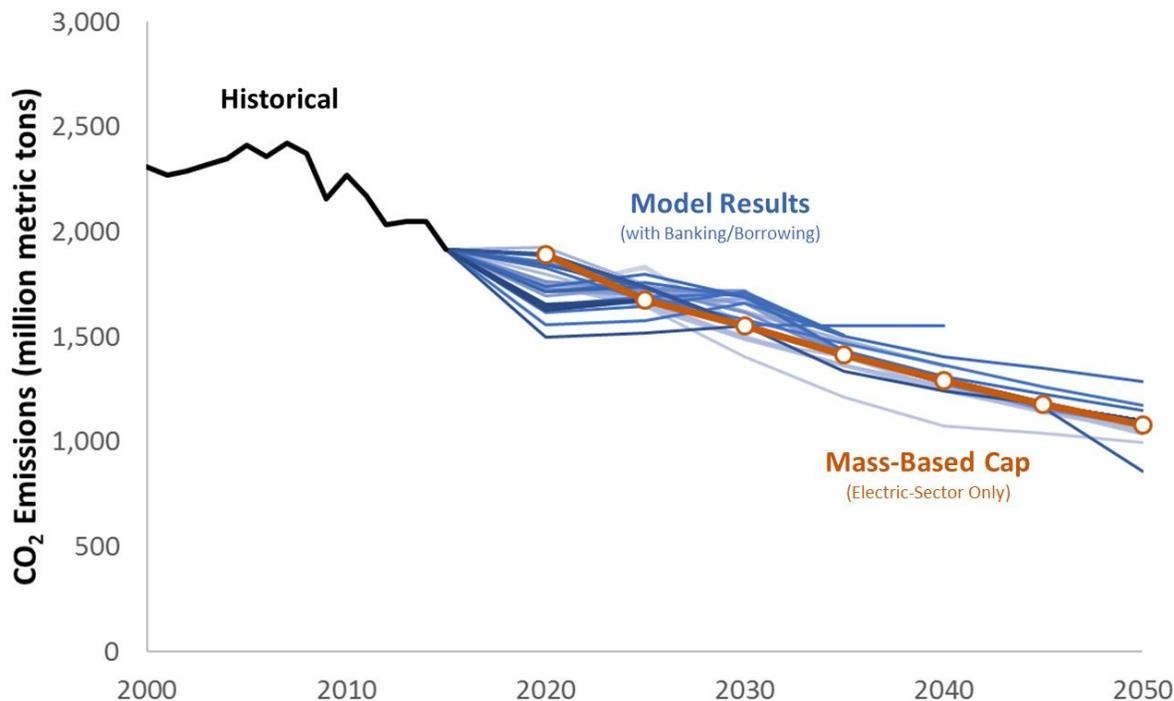
**Figure 22. Historical and projected U.S. electric sector CO<sub>2</sub> emissions (million metric tons) across models (2000–2050) under mass-based policy conditions.** Blue lines represent individual models, and the orange line shows the cap value (i.e., without banking and borrowing).
