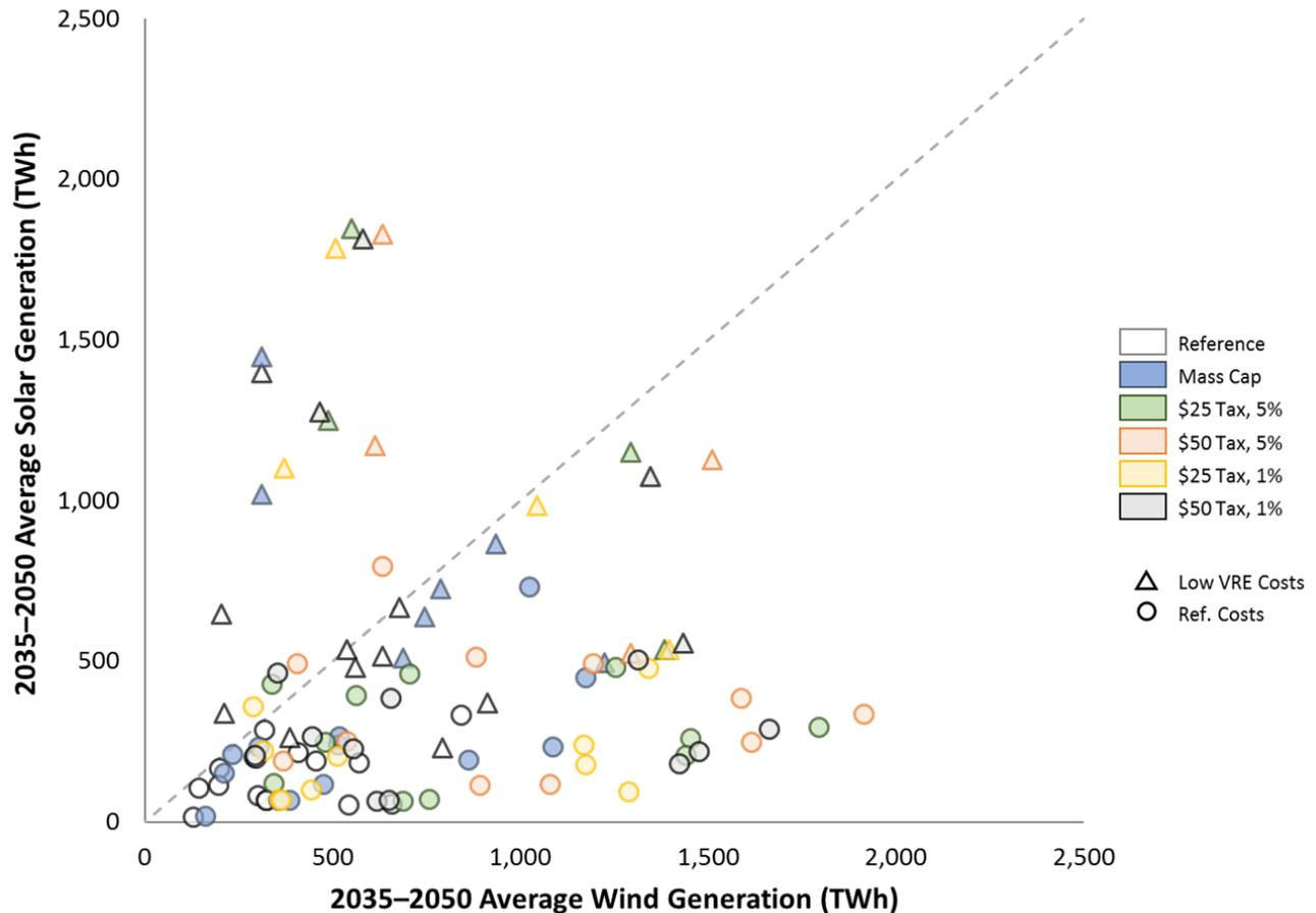
**Figure 5. Comparison of average annual U.S. wind and solar generation (TWh/yr) between 2035–2050 with reference and lower wind and solar costs.** Points represent individual model runs with colors corresponding to the policy scenarios. Reference wind and solar cost scenarios are represented by circles and lower-cost scenarios by triangles. Values above (below) the dotted line indicate higher solar (wind) generation for a given model and scenario.
