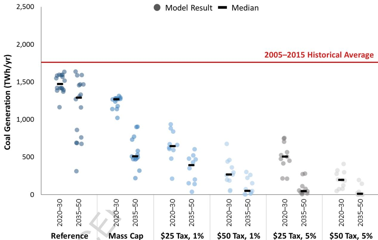
**Figure 15. Annual coal generation (TWh/yr) for all models and technology scenarios, grouped by policy scenario and time period.** Generation is the sum of all U.S. coal units without and with CCS. Values shown for the reference technological scenario only. Historical average generation from EIA (2016b).
