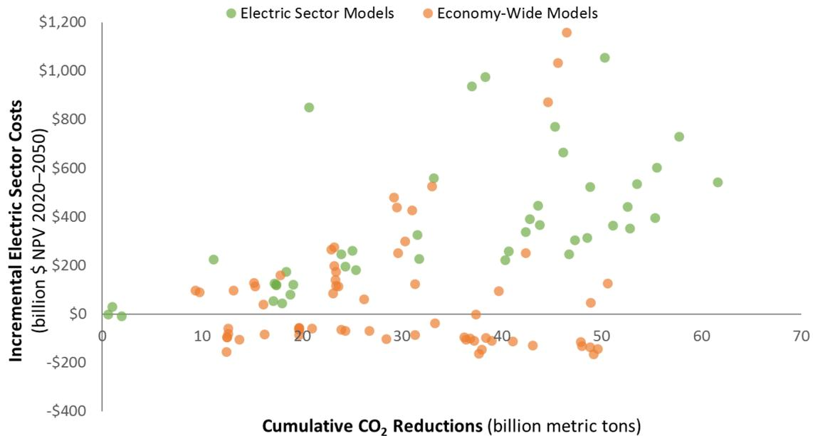
**Figure 13. Comparison of cumulative CO<sub>2</sub> reductions (billion metric tons) and incremental electric sector costs (billion \$ NPV 2020–2050) relative to the reference scenario.** Dots represent individual model runs. Green circles show electric-sector-only models, and orange values show economy-wide models. The average NPV under reference scenarios is \$2.77 trillion.
