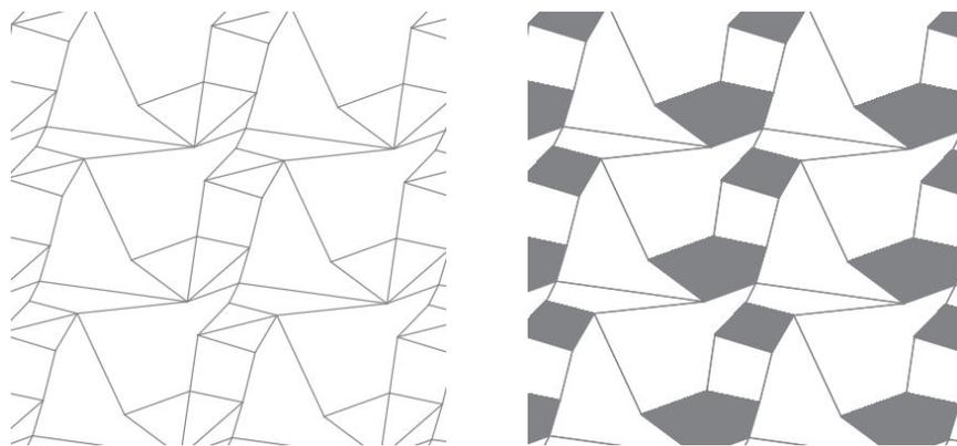
FIG. 2. *Left: A 2D periodic bar-and-joint framework containing smaller rigid components. Right: The same framework, viewed as a body-and-bar framework; the rigid components form the bodies, and the remaining bars connect distinct bodies.*
