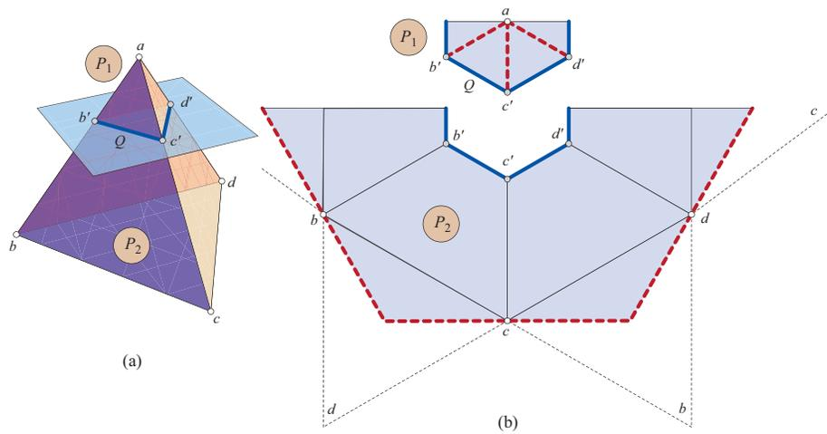
Figure 3: (a) Regular tetrahedron sliced at  $\frac{2}{3}$ 's of its altitude. (b) Unfoldings of  $P_i$ , with cut loci  $C_{P_i}$  drawn dashed.  $C_{P_2}$  partitions the bottom face  $\triangle bcd$  into three congruent triangles meeting at its centroid.
