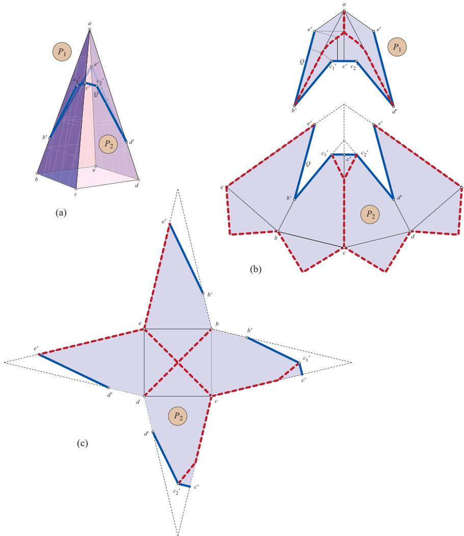
Figure 5: (a) A square-based right pyramid, with altitude twice the base side length.  $|bb'| = |dd'| = |ae'| = \frac{1}{4}|ab|$ , and  $|b'c'_1| = \frac{3}{4}|b'e'|$ . (b) Source unfolding of the two halves  $P_1$  and  $P_2$ . (c) A view of  $P_2$  from the bottom of the pyramid.
