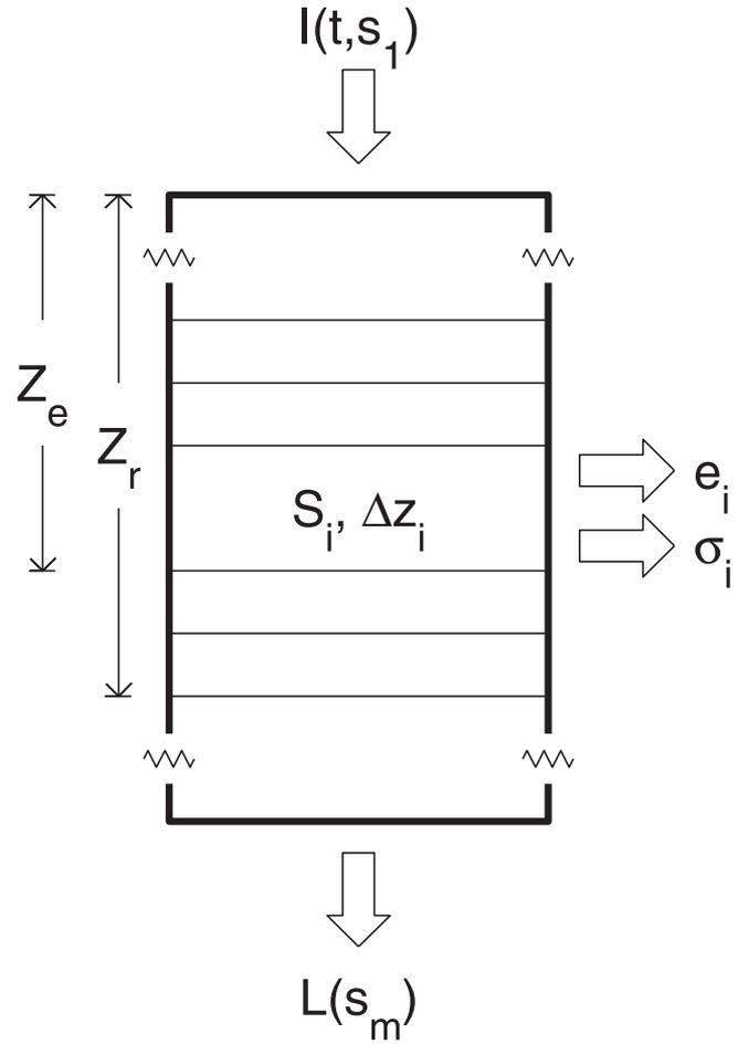
**Figure 3.** Schematic representation of the one-dimensional Richards model.
