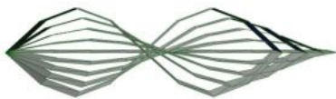
Figure 6: Isometric morph of a simple polygon. The start polygon is a 3D polygon obtained by discretizing the curve y = \sin(x) and by adding thickness to the curve along the z -direction. The end polygon is similarly obtained from y = -\sin x .
