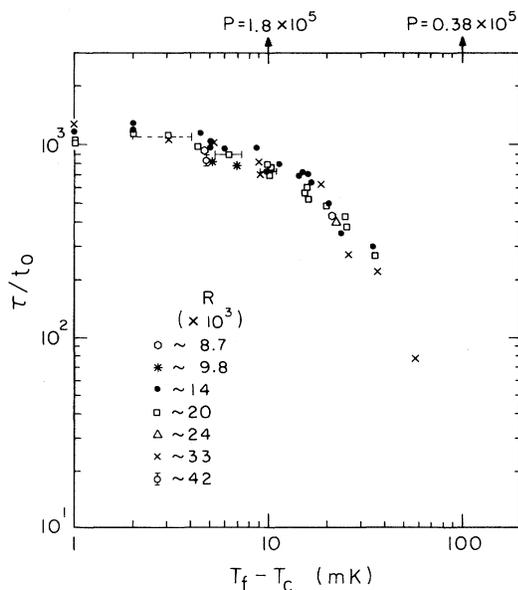
FIG. 1. Mixing time scaled by the turnover time  $t_0$  plotted as a function of  $T_f - T_c$ , for several different Reynolds numbers. All measurements have  $T_c - T_i = 150$  mK.  $P$  values are indicated on the upper scale.
