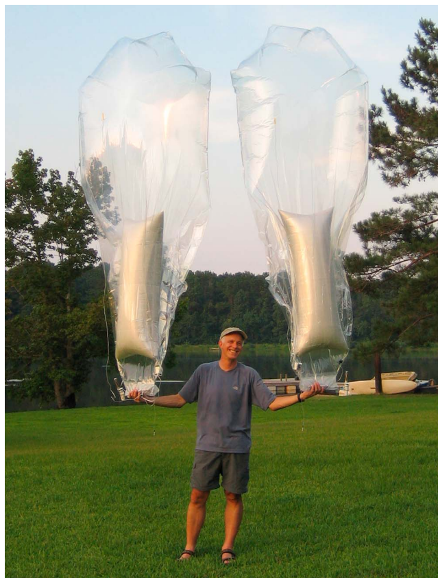
Figure 1. A pair of two CMET balloons just before launch from an open site north of Houston.
