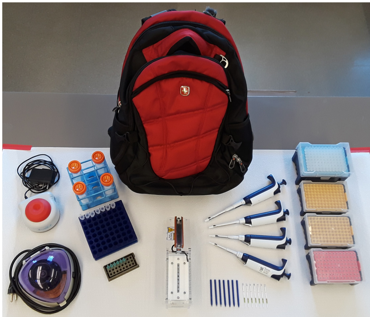
Fig 3. The contents of the “Backpack PCR” platform. The entire “Backpack PCR” platform weighs less than 10 lbs and can be easily transported by a single person. The “Backpack PCR” platform, which couples a simple and inexpensive NaOH-based extraction method with miniPCR amplification and test strip detection, will facilitate the use of molecular xenomonitoring in resource-limited settings. Furthermore, as this platform is based upon commercially available technologies, it will prove readily adaptable to the detection of W. bancrofti and other mosquito-borne pathogens. Research to develop this platform for the detection of other parasite and viral pathogens found in mosquitos is ongoing in our laboratory.
