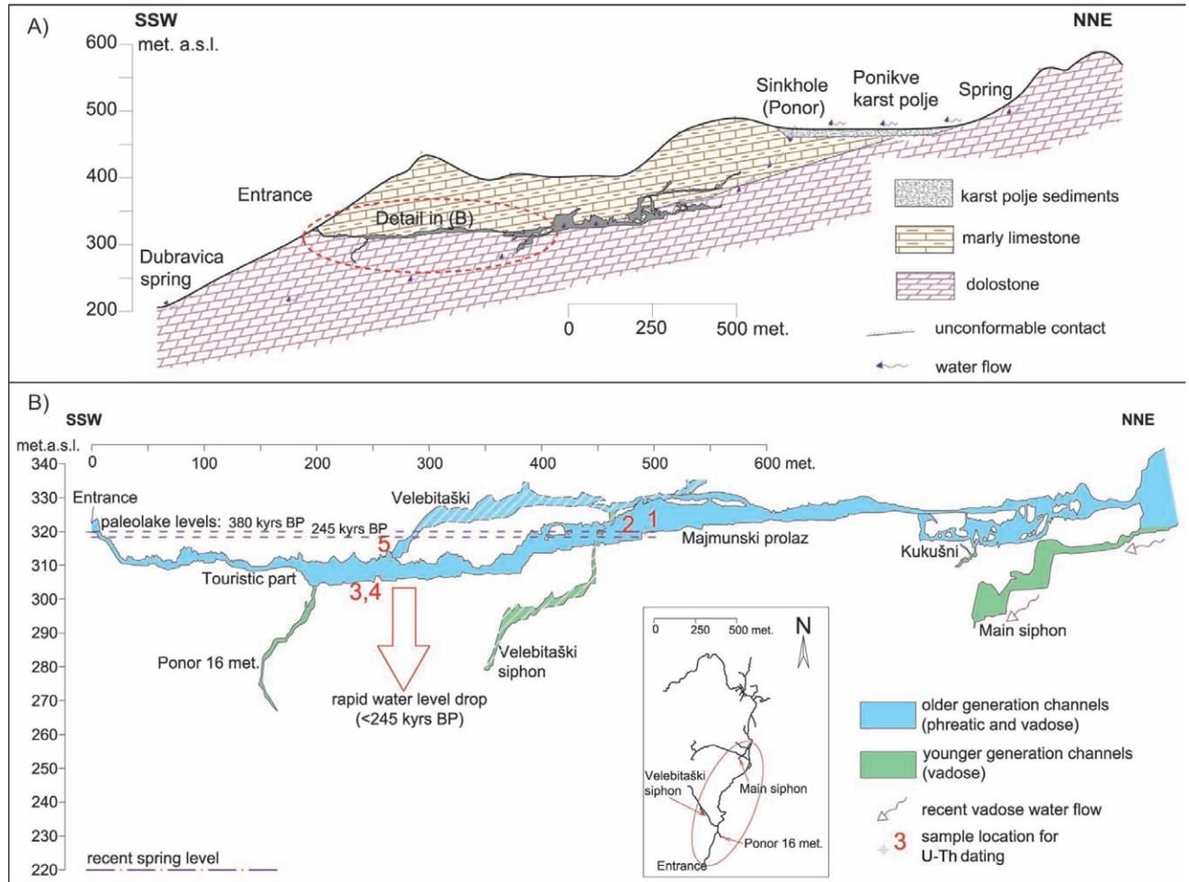
**Figure 2:** Cross-sections of the main Veternica Cave passages. A) Geological profile illustrating the water drainage pattern from sinkholes along the Ponikve karst polje and through the cave to the Dubravica spring. B) Enlarged area to show detail of the main cave passage and parts of the side channels. Shelfstone (1 & 2) and flowstone (3, 4 & 5) sampling locations are indicated. Reconstructed palaeolake are also shown. Note vertical exaggeration.
