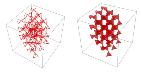
Figure 2: The quartz framework is an example of a tetrahedral 3D periodic structure. It has n=6 vertex orbits and m=3n=18 edge orbits. The barand-joint framework is shown on the left. The edges of the three highlighted tetrahedra provide the 18 representatives for the edge orbits. In [6], we show that the path of the phase transition from low to high quartz is auxetic.
