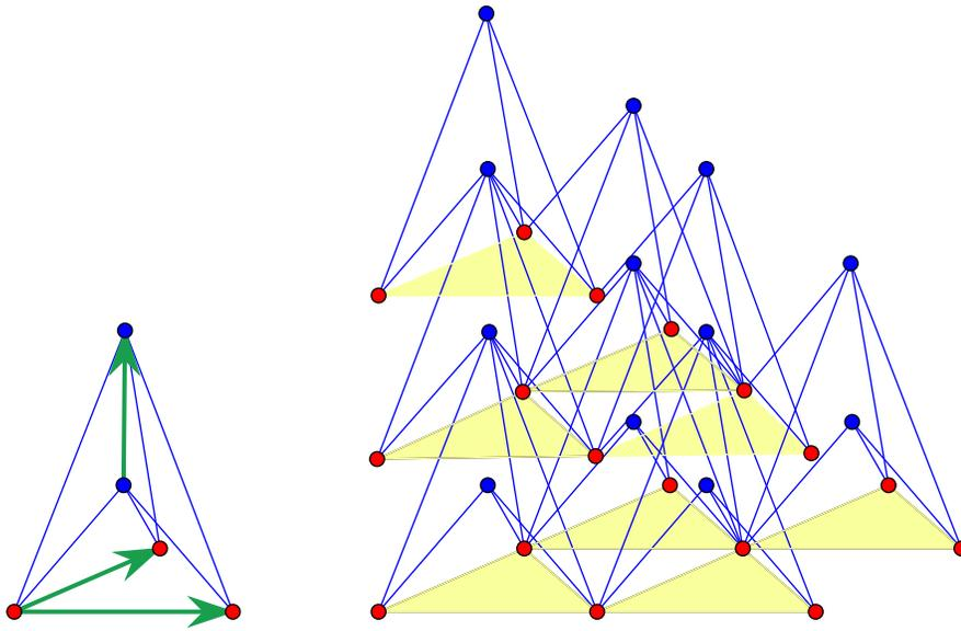
**Figure 7.** A finite linkage in  $\mathbb{R}^3$ , with 5 vertices, 6 edges, and 3 pairs of vertices marked by arrows. A fragment of the associated periodic framework is shown nearby. It has 2 orbits of vertices and 6 orbits of edges modulo periodicity.
