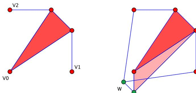
**Figure 8.** The planar linkage in Figure 5 has two degrees of freedom but can be converted into a single degree of freedom mechanism which retains the desired infinitesimal deformation on the vertices  $v_0, v_1, v_2$ .
