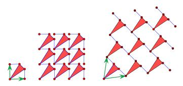
**Figure 5.** A finite linkage with two degrees of freedom with auxetic capabilities for the associated periodic framework. The deployed configuration on the right can be reached via an auxetic path.
