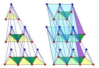
**Figure 10.** Auxetic mechanism. The fragment shows three floors. We show an alternative view as "breathing stacked roofs." Inhaling is auxetic. The one degree of freedom deformation can be parametrized by the dihedral angle of a roof. The floors vary accordingly. The framework edges are all contained in roof planes. Floors contain no edges but must respect periodicity constraints.
