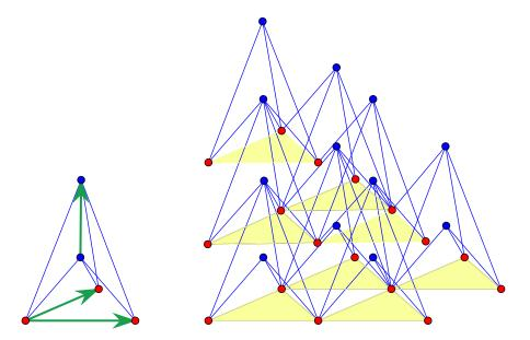
**Figure 7.** A finite linkage in  $\mathbb{R}^3$ , with 5 vertices, 6 edges, and 3 pairs of vertices marked by arrows. A fragment of the associated periodic framework is shown nearby. It has 2 orbits of vertices and 6 orbits of edges modulo periodicity.
