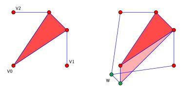
**Figure 8.** The planar linkage in Figure 5 has two degrees of freedom but can be converted into a single degree of freedom mechanism which retains the desired infinitesimal deformation on the vertices  $v_0, v_1, v_2$ .
