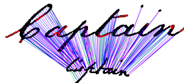
Fig. 1. Alignment of one image with a second (shown to scale). Areas with red dots have no match detected in the opposite image.
