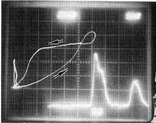
FIG. 3. Switch-off in a 12- $\mu\text{m}$ -thick CuCl etalon. When the input dye-laser pulse (right) is adjusted for a slow falloff, switch-off in the output pulse (center) is clearly seen. The time scale is 5 ns/div.
