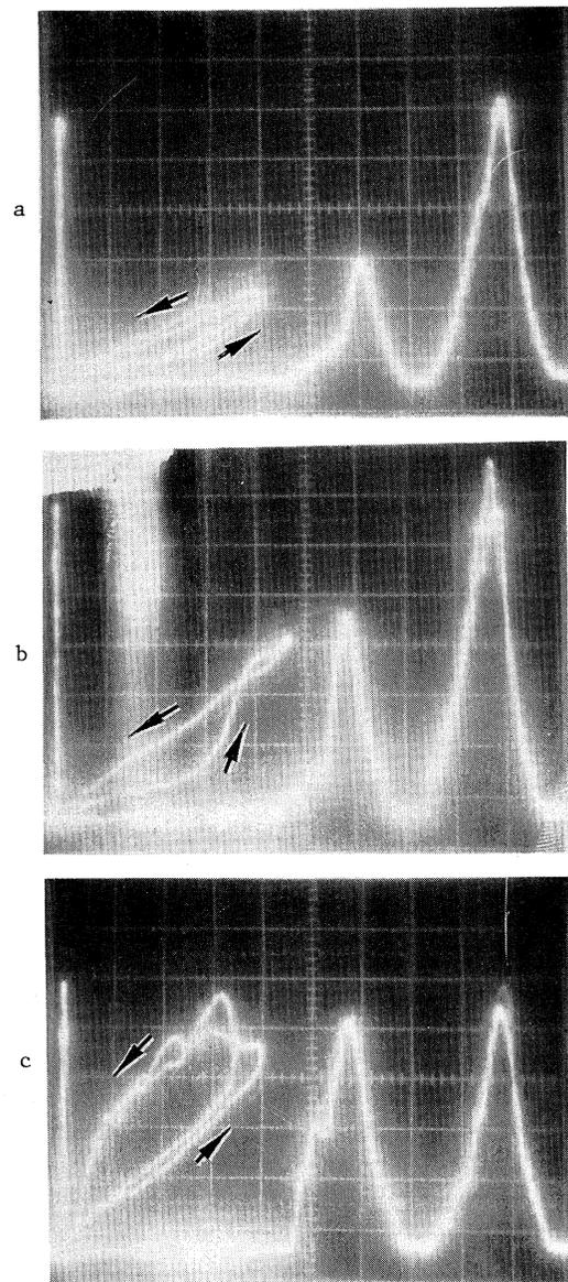
FIG. 2. Switch-on in a 12- $\mu\text{m}$ -thick CuCl etalon. The laser frequency is gradually increased (corresponding to a fraction of a millielectronvolt change) in the sequence of photographs (a)–(c). Each photograph shows hysteresis loop, output pulse (center), and input pulse (right). Note that only (b) shows switch-on. Switch-off is not resolved in (b) as the input dye-laser pulse falls too steeply. The time scale is 5 ns/div.
