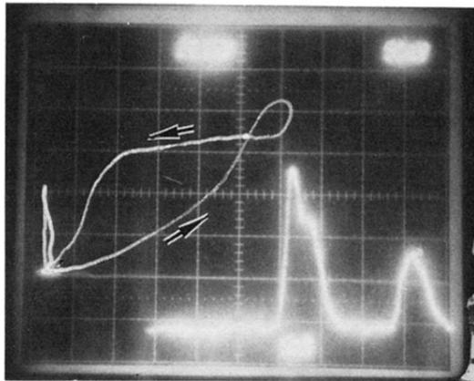
FIG. 3. Switch-off in a 12- $\mu\text{m}$ -thick CuCl etalon. When the input dye-laser pulse (right) is adjusted for a slow falloff, switch-off in the output pulse (center) is clearly seen. The time scale is 5 ns/div.
