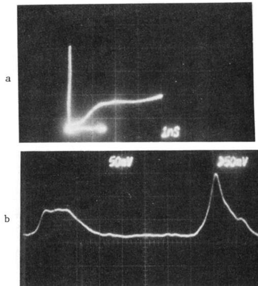
FIG. 1. Limiting action in a  $10\text{-}\mu\text{m}$ -thick CuCl etalon. (a) Output vs input intensity. (b) Input pulse (right) and output pulse (left) vs time.
