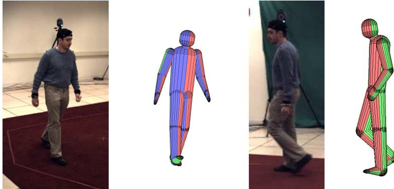
Figure 6: Sample erroneous reconstructions. A small slide occurs on *S2-Combo-1-C1* around frame 100 (left). Poor initialization causes a reversal on *S2-Combo-1-C3*, shown right at frame 114. The reversal is corrected soon after via a stutter-step.
