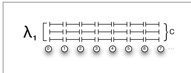
Fig. 1. Each node has a lightpath to the nodes immediately to its left and right.
