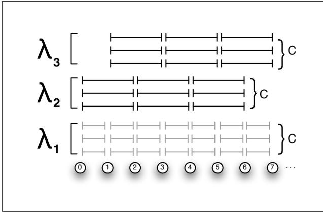
Fig. 2. Each node now has a lightpath to its neighbors at distance 2, using the next pair of wavelengths.
