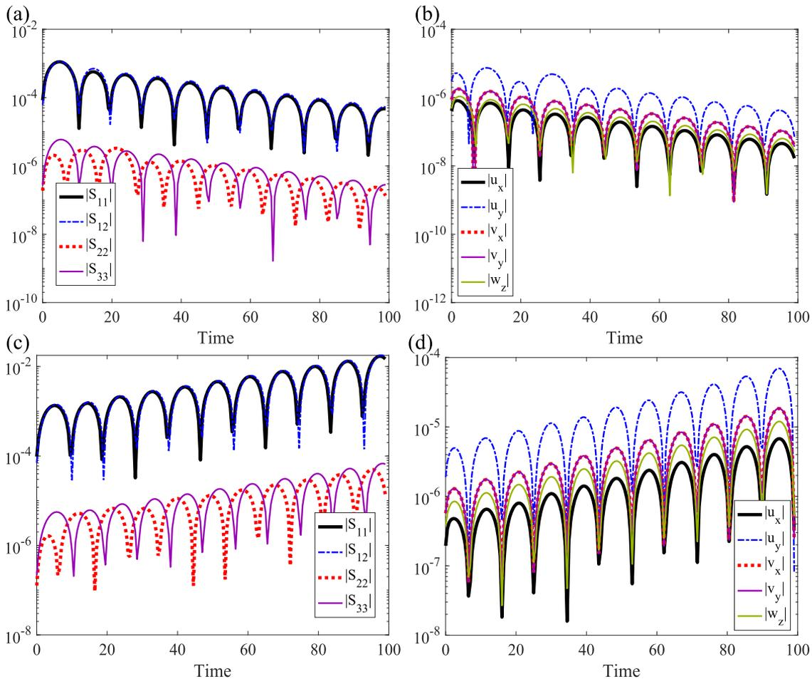
FIG. 15. (a) and (b)  $Wi = 8$ , (c) and (d)  $Wi = 12$ . Temporal evolution of linear perturbation for  $|\tilde{S}_{11}|, |\tilde{S}_{12}|, |\tilde{S}_{22}|, |\tilde{S}_{33}|, |\partial_x \bar{u}|, |\partial_y \bar{u}|, |\partial_x \bar{v}|, |\partial_y \bar{v}|, |\partial_z \bar{w}|$  at  $(\pi, \pi, 0)$ .
