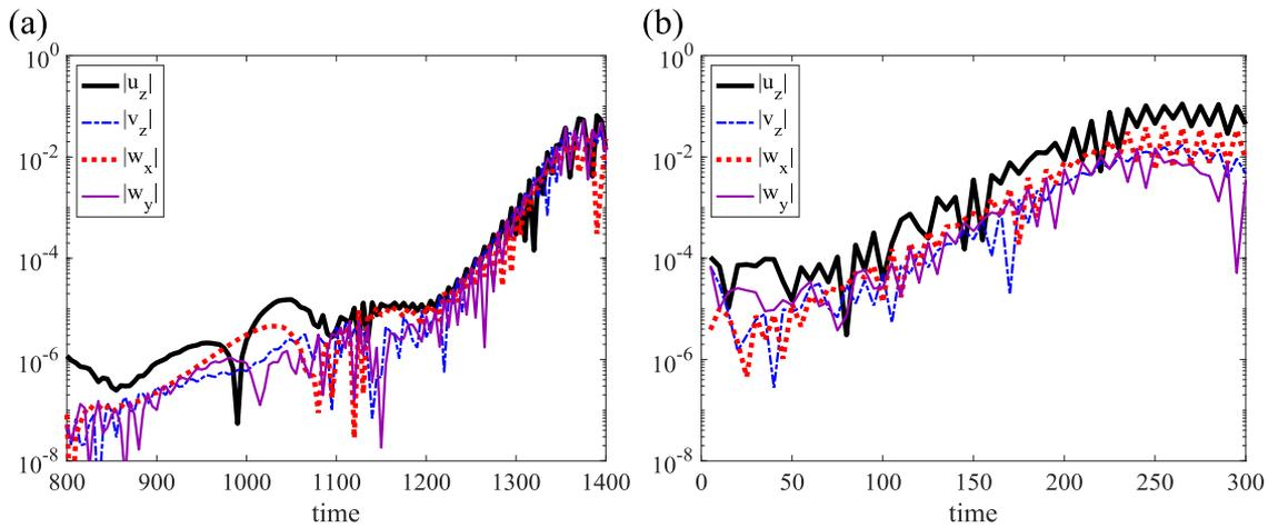
**FIG. 11.** Data from Oldroyd-B simulation described in Secs. III B 1 and III B 2 for (a)  $Wi = 8$  and (b)  $Wi = 12$ . Temporal behavior of  $\partial_z u, \partial_z v, \partial_x w, \partial_y w$  at  $(x, y) = (\pi, \pi)$  for  $z = 0.88$ ; note the log scale on the y-axis. These are components of the velocity gradient that are zero when there is no  $z$ -dependence in the flow.
