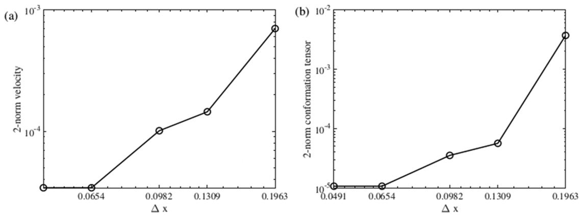
FIG. 2. Grid refinement study. Errors computed by comparing with the finest resolution  $N = 192$ , (a)  $L^2$  norm of the velocity, (b)  $L^2$  norm of the conformation tensor.
