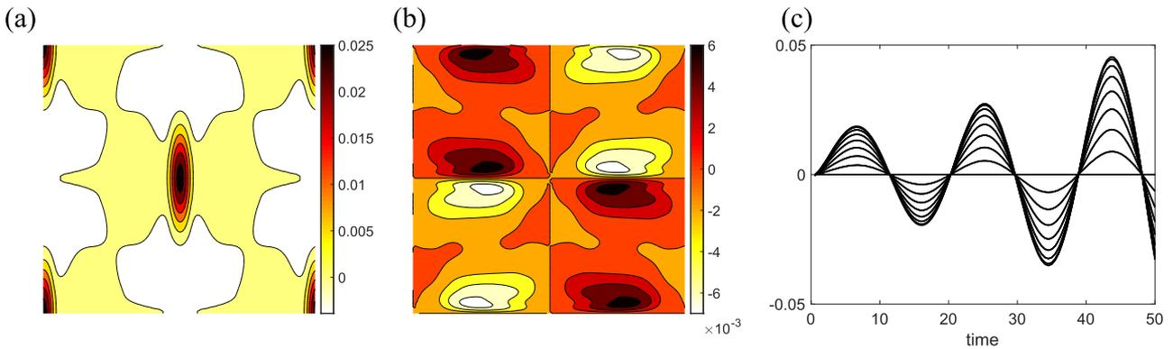
**FIG. 12.** Solutions from linear evolution of the Oldroyd-B system with  $Wi = 12$ . (a) Contours of  $\tilde{S}_{13}(x, y, \pi/2, t_e)$  for  $t_e = 24.5$ , (b) contours of  $\tilde{S}_{23}(x, y, \pi/2, t_e)$  for  $t_e = 24.5$ , and (c)  $\tilde{S}_{13}(\pi, \pi, z, t)$ , for several locations  $0 < z < \pi$  and  $Wi = 12$ .
