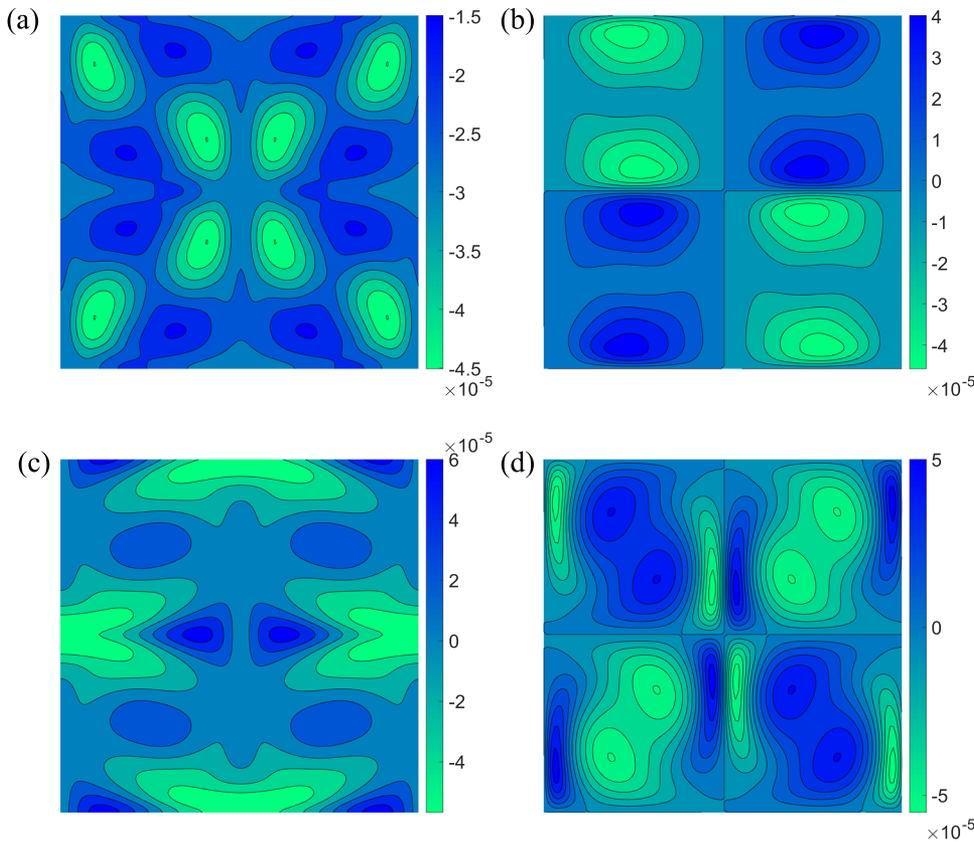
**FIG. 13.** Components of the velocity gradient at  $t_e = 24.5$ ,  $Wi = 12$ . (a)  $\partial_z \bar{u}(x, y, \pi/2, t_e)$ , (b)  $\partial_z \bar{v}(x, y, \pi/2, t_e)$ , (c)  $\partial_x \bar{w}(x, y, \pi/2, t_e)$ , and (d)  $\partial_y \bar{w}(x, y, \pi/2, t_e)$ .
