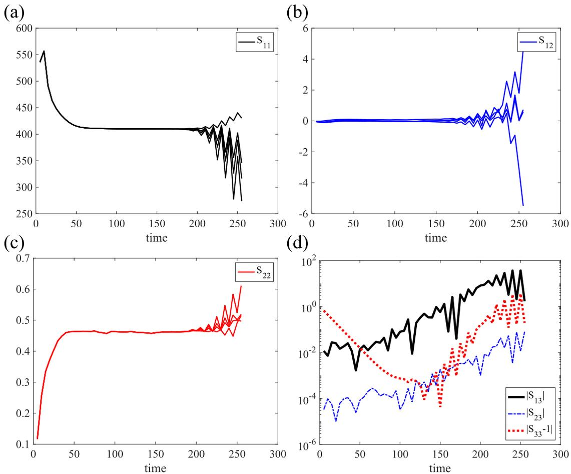
**FIG. 10.** Data from Oldroyd-B simulation described in Sec. III B 2 for  $Wi = 12$ . Temporal behavior of (a)  $S_{11}$ , (b)  $S_{12}$ , and (c)  $S_{22}$  components of the conformation tensor at  $(x, y) = (\pi, \pi)$  plotted at 4 different  $z$  values between 0.88 and 3.14. (d) Temporal behavior of  $|S_{13}|$ ,  $|S_{23}|$ ,  $|S_{33} - 1|$  components of the conformation tensor at  $(x, y) = (\pi, \pi)$  for  $z = 0.88$ ; note the log scale on the  $y$ -axis.
