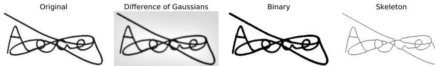
Figure 1: Image processing for keypoint graph shown on first signature of user 3902 from the GPDSsynthetic dataset [31].
