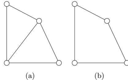
Figure 1: Bar-and-joint structures in two-dimensions: (a) minimally rigid and (b) flexible.
