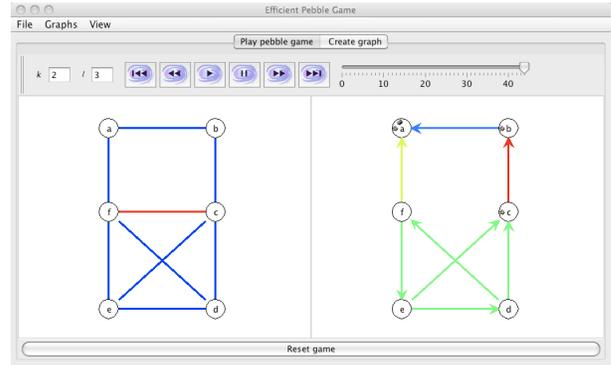
**Figure 4:** A snapshot of the component pebble game for 2D bar-and-joint rigidity.
