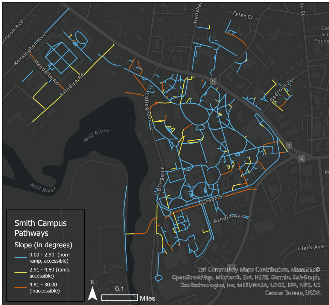
Figure 6: A map displaying slopes of paths around campus. Blue and yellow paths are both considered accessible slopes under the ADA, but orange slopes are too steep to be accessible under the ADA.
