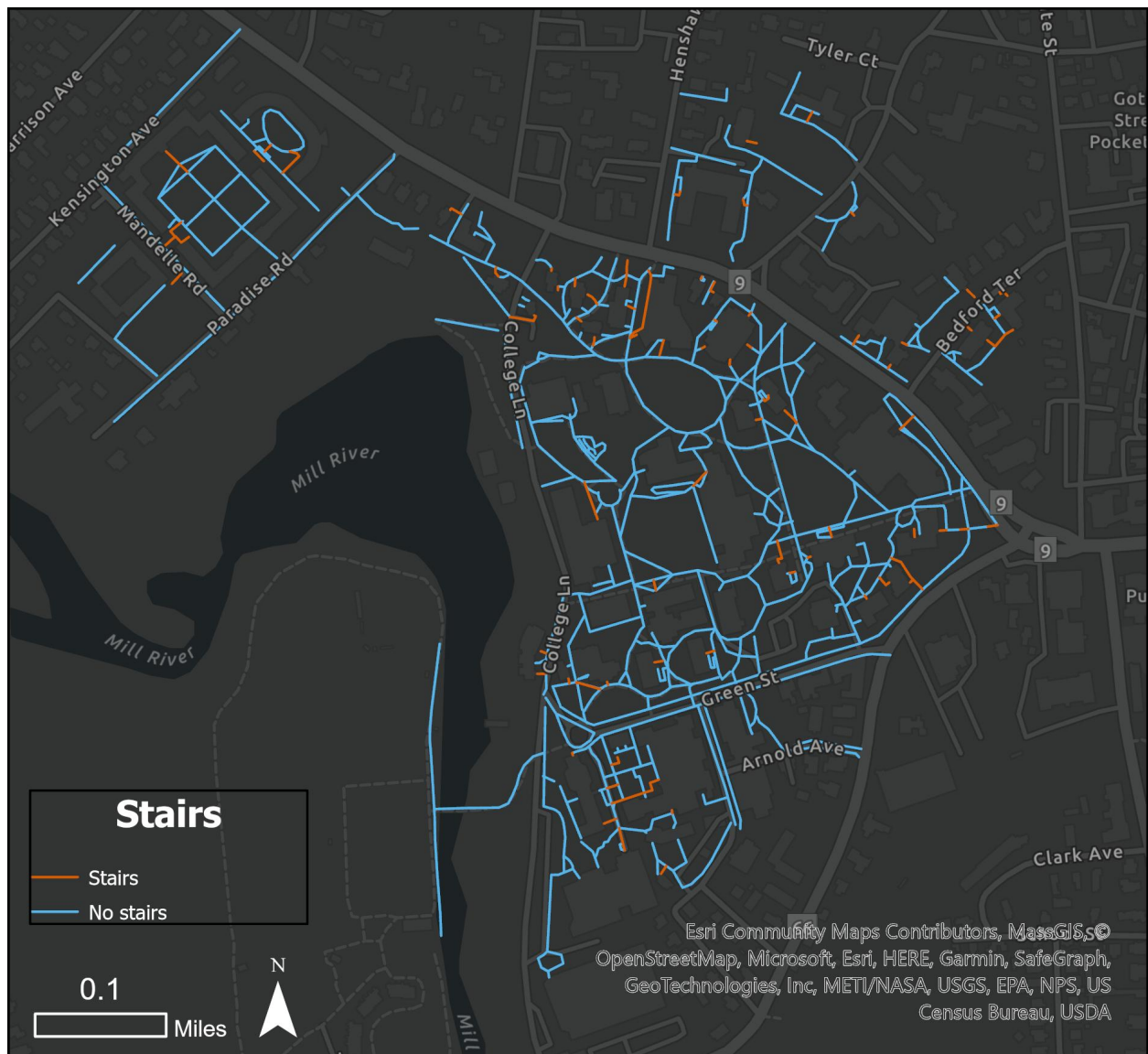
Figure 12: A map showing which paths have stairs (orange) and which do not (blue) of the paths we took data for.
