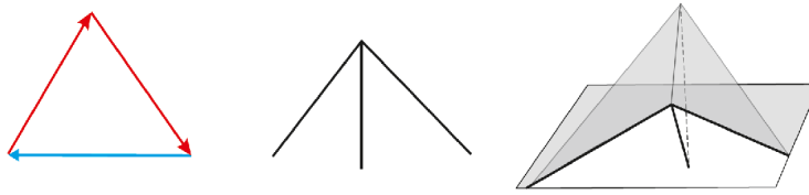
Figure 27: A virtual polytope represented by a colored chain (left), its fan (middle), the graph of its support function (right). In this particular case, the fan is not convex.
