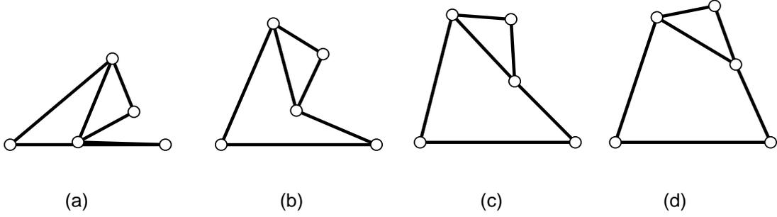
Figure 18: Four snapshots from the lifetime of a 1dof mechanism: (a) and (a) are the limit situations of of (b), which is expansive. (d) is not expansive: some diagonals increase, some decrease. Notice the change in the combinatorial structure from (b) to (d), via (c).
