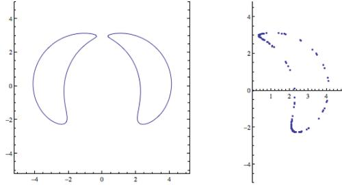
**Fig. 3** The singularity curve for a 2R manipulator, obtained after computing all coefficients of the degree four equation from sample points illustrated nearby.
